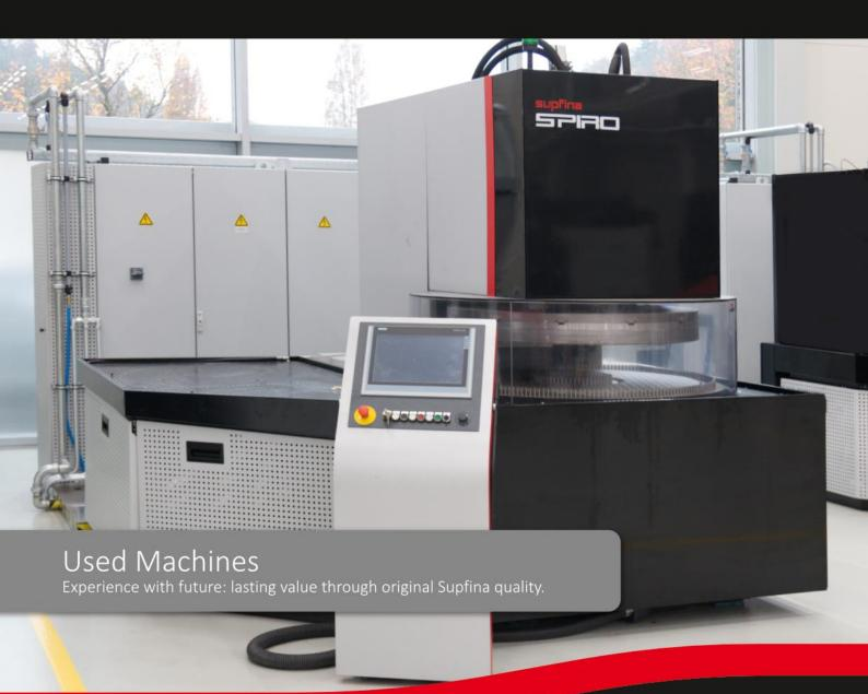
Fine grinding machine for high-precision and economical machining of large workpieces
